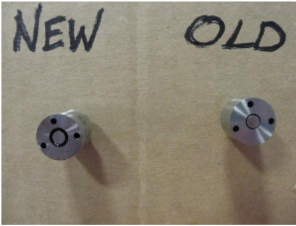
Here you can see the difference between the newer style nozzle and the older style nozzle. Take note of what you have when removing your parts.
