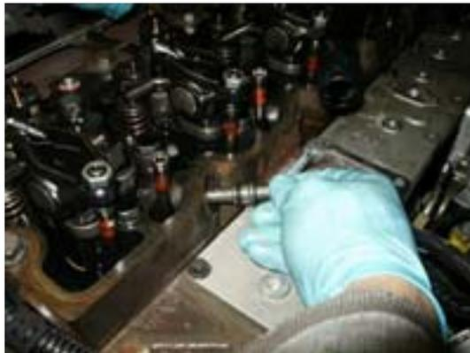
33: Replace connector tube nuts and finger tighten.
