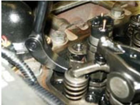
24: Use Supplied injector hold tool to secure injector in a vise. The tool fits between the two loose collars on the injector.
