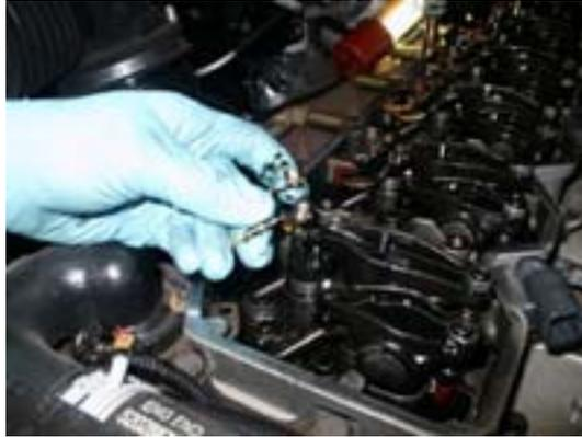
7: Remove 10mm bolts holding riser box.
