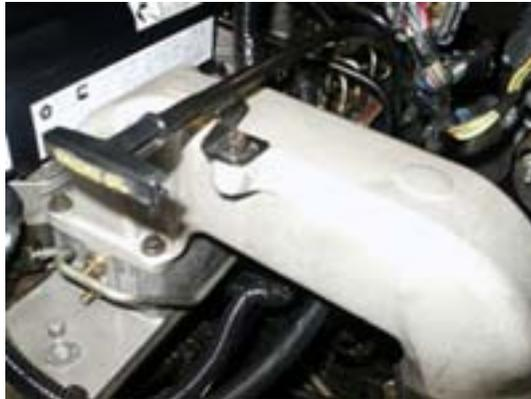
3: Remove 11mm Intercooler boot clamp.
