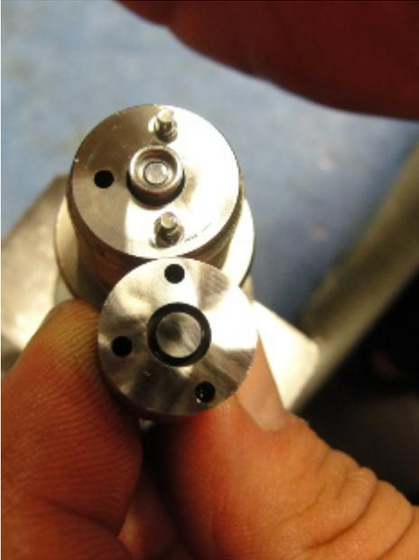
This is the new style nozzle and injector body. Here you can see the “collar” that fits up inside the updated nozzle assembly.
