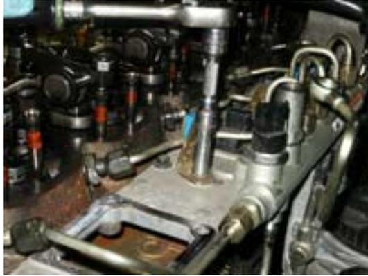
16: Remove 10mm bolts holding fuel rail.
