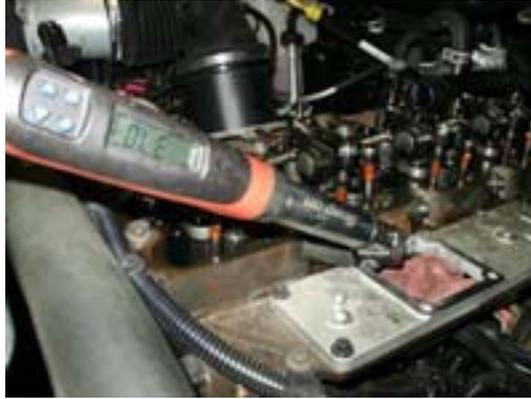
36: Torque injector hold down nuts to 89in. lbs.
