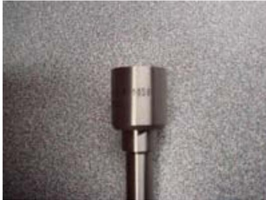
28: Inspect nozzle for cracks. The whit arrow above shows a nozzle that was crazked by elevated rail pressure from a downloader, chip or module. If you have a cracked nozzle, you must buy a new injector since it will be cracked as well.
