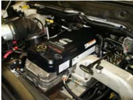
57: Reconnect negative battery cables, and start truck. There will be some smoke at startup that should go away within 30 seconds or so. If the truck does not start check connector tube torque. Under no circumstances should the high pressure fuel lines be loosened to bleed. The system is self bleeding. You can be maimed or killed.
