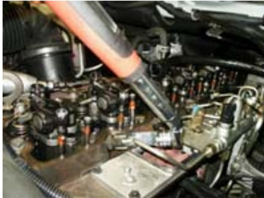
43: Install fuel line hold down bracket at rear of fuel rail, and torque to 18ft lbs.
