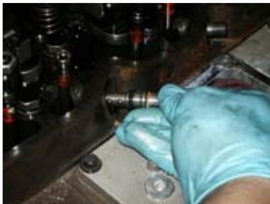
22: Remove 8mm injector hold down bolts.
