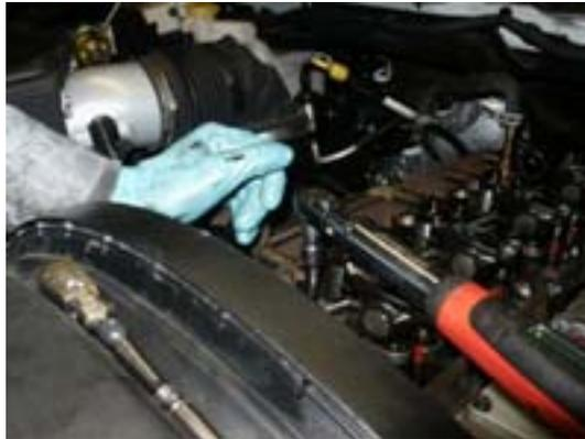
37: Reinstall engine lift bracket torque to 57ft lbs.
