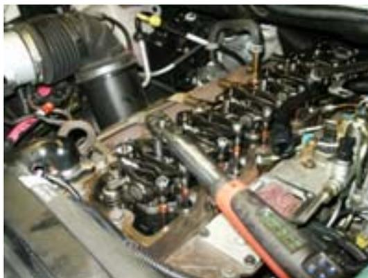
49: Install riser box, and torque to 18ft lbs.
