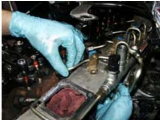
40: Connect high pressure supply line, and finger tighten.
